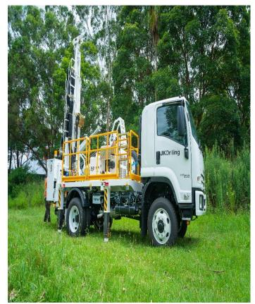
The Compact Rig – 4 x4 truck mounted multipurpose rig, ideal for safe and efficient auger, rotary or cored boreholes
